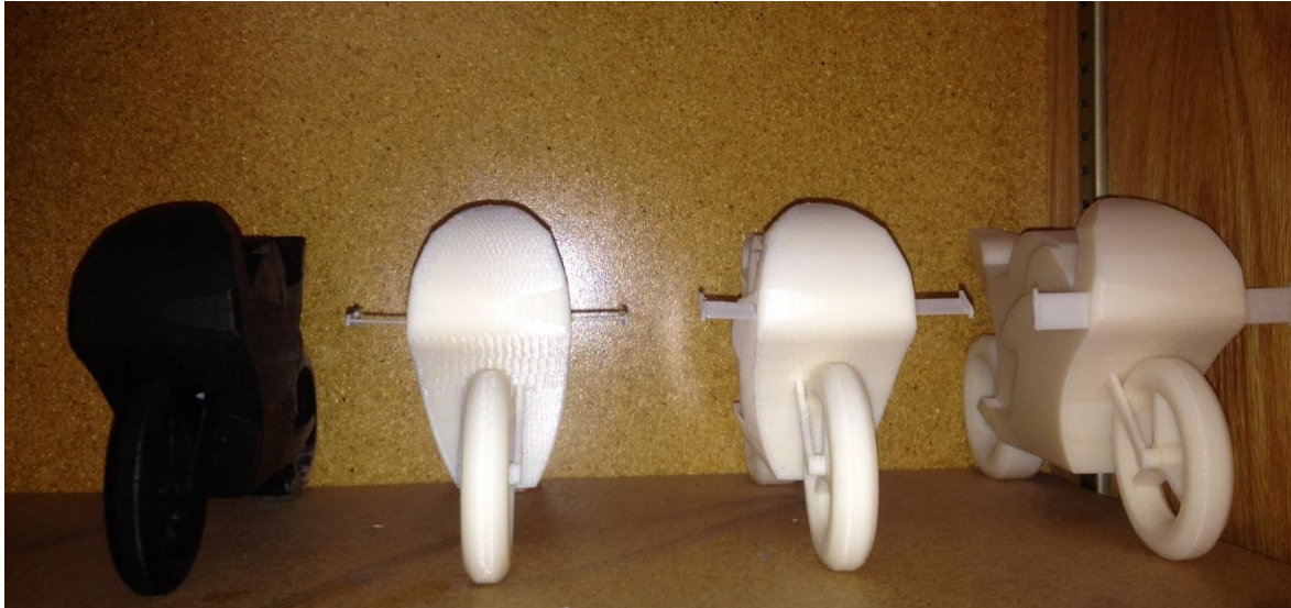
Figure 20. Finalized 3D Printed Models. FROM LEFT: Non-Wing, 0 Degrees, 10 Degrees and 90 Degrees Models.
