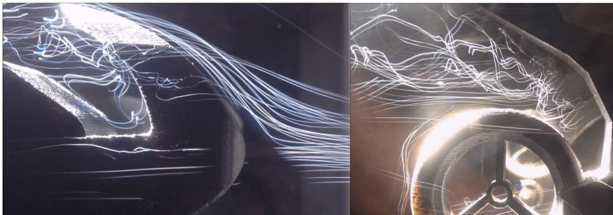
Figure 21. Visualization Testing using the Wind Tunnel. LEFT: Headlamp area showing the flow separation, the stagnation point and vortices behind the windblast area. RIGHT: Tail end vortices a.k.a. Wake of the Motorcycle.
