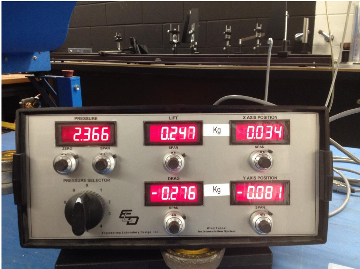
Figure 30. Non-Wing Prototype Gauge Indication at 44.7m/s i.e. Test Wind Speed.
