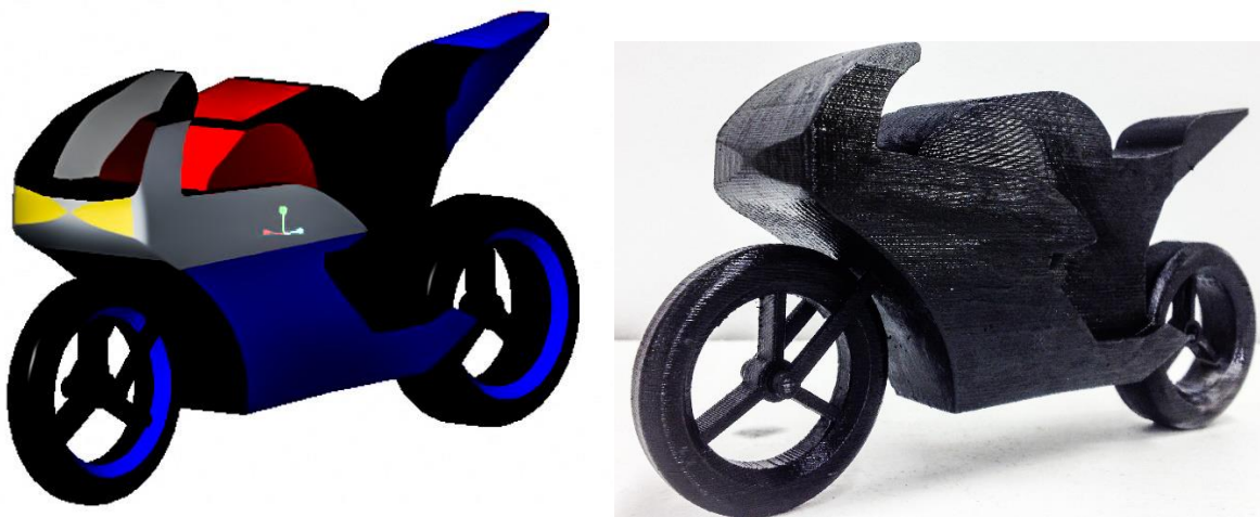
Figure 4. Comparison between a Mathematical (CAD) Model and a Physical Model.
