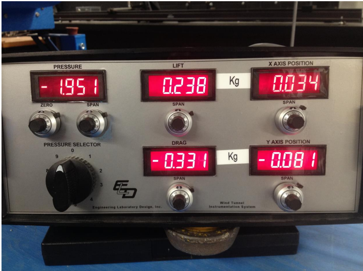
Figure 35. 90 Degree Wing Prototype Gauge Indication at 44.7m/s i.e. Test Wind Speed.
